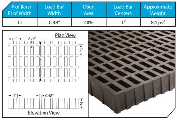
Section Properties per Ft of Width: A = 10.26 IN<sup>2</sup> I = 3.4 IN<sup>4</sup> S = 3.27 IN<sup>3</sup>
