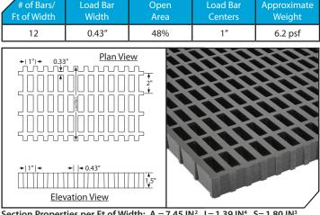
Section Properties per Ft of Width: A = 7.45 IN<sup>2</sup> I = 1.39 IN<sup>4</sup> S= 1.80 IN<sup>4</sup>
