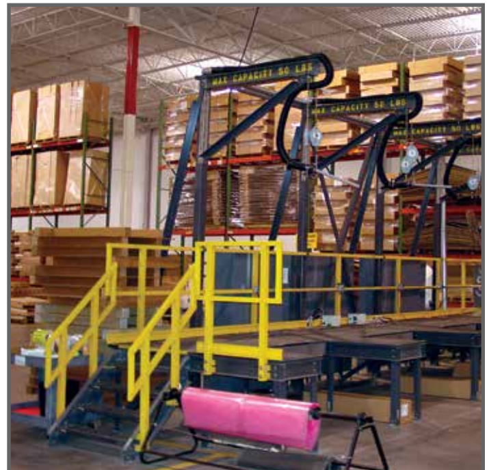
FRP products were chosen to upgrade these computer mainframe packaging platforms from wood.
