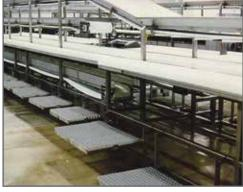
Photo Above: FGI-AM® grating was utilized for work station platforms that could adjust to the height of the line workers.
