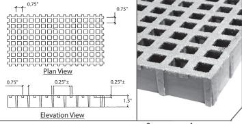
Section Properties per Ft of Width:  $A = 2.85 \text{ IN}^2$   $I = 0.51 \text{ IN}^4$  S = 0.65
