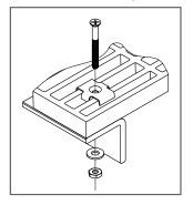
This 62% open area molded grating does require an E-1 Clip Assembly (shown above) to secure the grating to a structure. The WLP Clip Assembly will also work.
