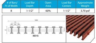
Section Properties per Ft of Width:  $A = 3.23 \text{ IN}^2$   $I = 0.95 \text{ IN}^4$   $S = 1.23 \text{ IN}^3$ Average EI = 5,870,707 lb - in<sup>2</sup> (SPAN  $\ge 30''$ )
